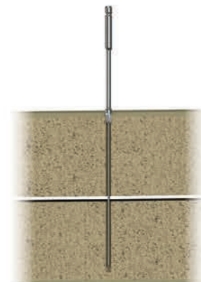
Figure 4 Countersinking a recess for the screw
